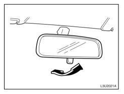
The day/night adjustment allows you to adjust the mirror to avoid glare from any headlamps behind you. Push or pull the tab for daytime/night use.
